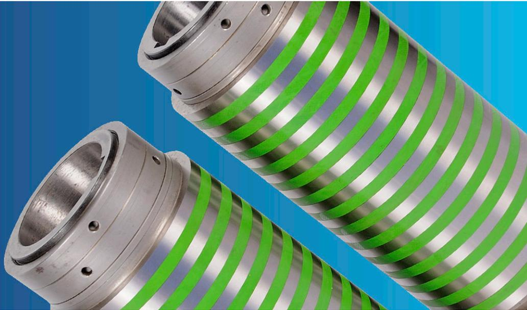
*Z.C. Quills are pre-assembled cutting sets made up of circular knives, metallic spacers and vulcanized spacers. Their main application is for cutting great tonnages of slit strips which are thin and have fixed widths.. Even more the higher the quality requirements are. These complete units remain assembled from the moment they are mounted, during their successive sharpening and until the end of their useful cutting life.*
